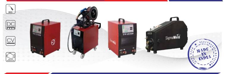
Sigmaweld series welding machines are sophisticated IGBT based inverters with total digital control having wide current range.
