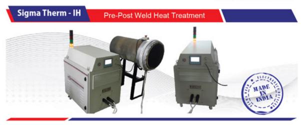
The Sigma Therm is an inverter based preheating and post weld heat treatment unit especially for tubes and pipes. Depending on the size of the pipe, one or two units are used. Induction coils are placed on both the sides of the welding seam.
