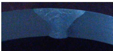
Figure 1 Penetration Profile of 8.5mm thick tube single pass welding with S.W.A.T
