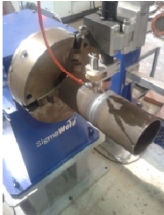
Auto GTAW with AVC, Weaving and Cold wire feeder Setup
